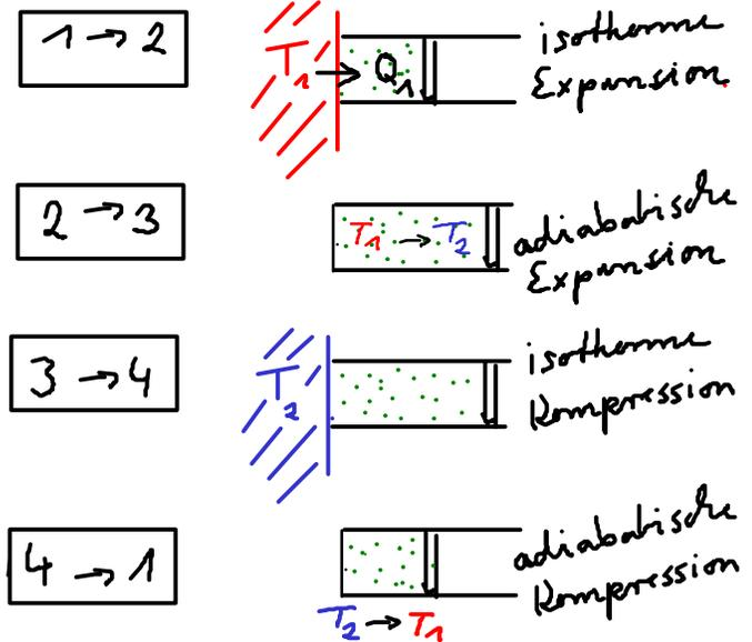
1 → 2       $V_1 \rightarrow V_2$        $\Delta T = 0$
